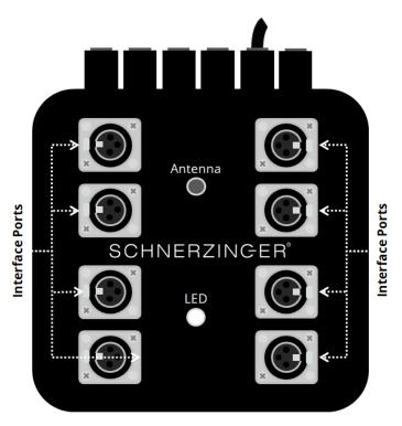
For each single component please test the optimal input; primary digital inputs, alternatively analog inputs. Per component only one INTERFACE will be connected. If the right and left channels are available for analog inputs, one channel will be connected via an INTERFACE, while the second channel may be connected to a GIGA GUARD. If no digital or analog input is available, the effect of an INTERFACE may also be tested at an output (digital or analog, but no speaker terminal\*).
